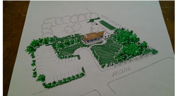
**Figure 1: Illustration of proposed new meeting room design, to be connected to the existing building via a welcoming room. This design improves the arrival sequence and uses expenses more efficiently.**
